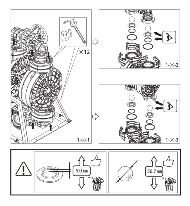
**2**-② **2**-① AC AN AE AV AT AH AS FC FN FE FV FT FH FS SC SN SE SV ST SH SS 14mm 17mm ×16 ×16 2-①-1 2-2-1 2-12-2 2-12-3 2-12-4
