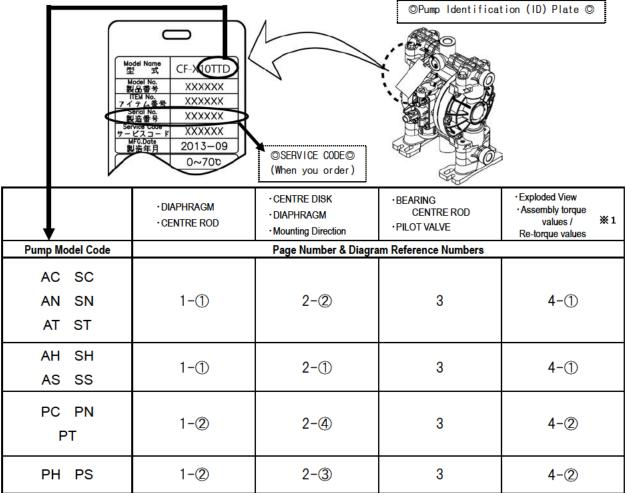
X 1 )Before operating the pump for the first time please re-torque all bolts. Also re-torque bolts if leaks are discovered as part of the daily inspection regime.
